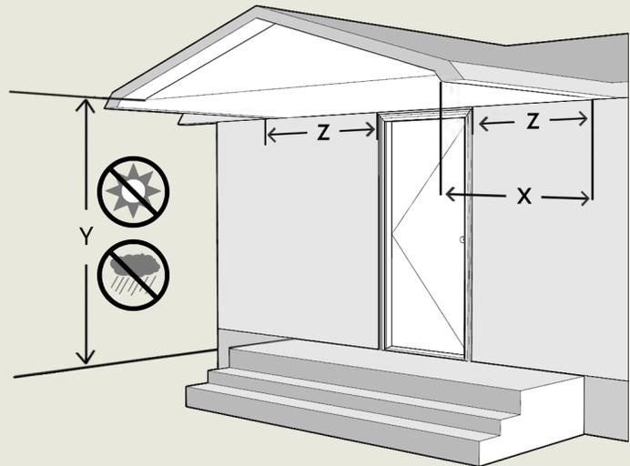
For detailed guidelines on the required overhang dimensions based on your door's specific orientation, please refer to the Overhang Requirements Diagram below. This diagram offers a clear visual representation of the necessary overhang measurements needed to ensure your door is adequately protected from direct environmental elements.
